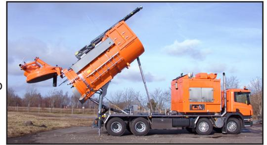
The unit is equipped with a separate diesel engine, offering the possibility to utilize local fuel taxation regulations. It also makes the machine's operation independently of the truck.
