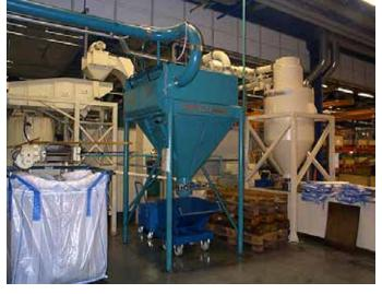
BEASS is the reliable and robust filter separator that fits most industries. The separator is equipped with the vacuum-controlled filter cleaning system ATM (re-pulse cleaning).
