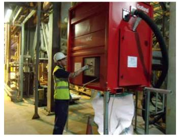
DISAB BagVA $C^{\text{TM}}$  is optimal for temporary suction needs such as cleaning, collection of spilt material or recycling of various materials.
