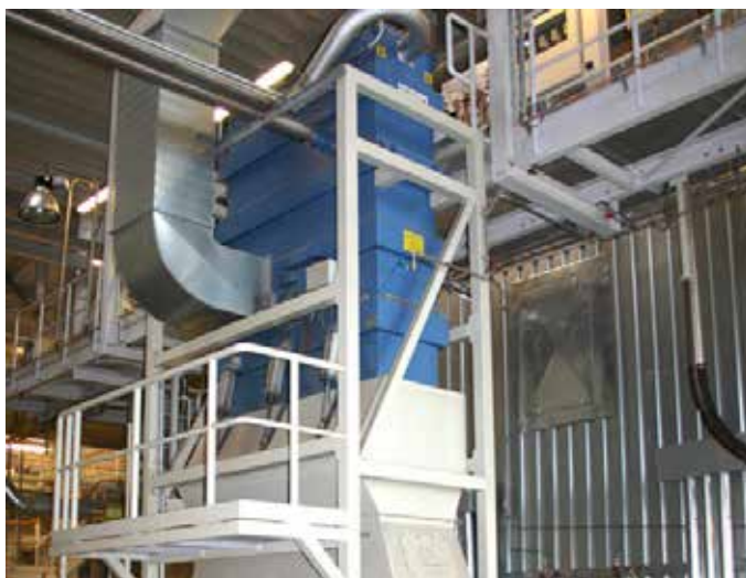
BEAT is the reliable and robust filter separator that fits most industries. The separator is equipped with the vacuum-controlled filter cleaning system ATM (re-pulsing cleaning).
