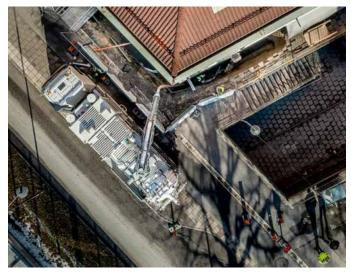
The vacuum unit consists mainly of a machine house and a container. The stable design and weight mean that the vacuum extractor must be handled by a four-axle hooklift truck.
