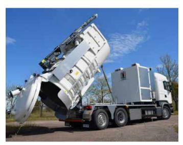
Emptying of the extracted material is easily done by tipping the tank and tailgate using a double-acting hydraulic cylinder.
