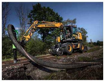
The unique mobility of the vacuum significantly streamlines train maintenance work. DISA-RAIL 1700 moves with ease on and off the track and on public roads. The ECORAIL MPC 30 is optimized for road transport, towed behind a tractor or truck.
