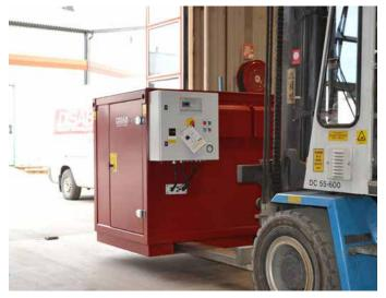
DISAB PES-101 comes with a complete control cabinet, which includes all equipment for easy use. With the help of the built-in fork aisles and lifting loops, you can easily move the vacuum unit, using a forklift or crane.
