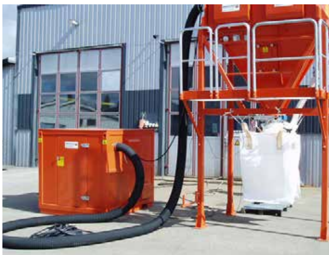
DISAB PES-7 units are a series of complete standalone vacuum units, intended for use with one of our filter separators.
