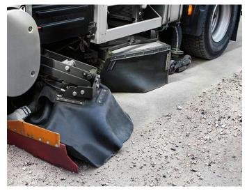
Due to the fact that the operation takes place completely without water, no contaminants are flushed out into the stormwater system and no contaminated sludge with the fine-grained dust remains on the road surface.
