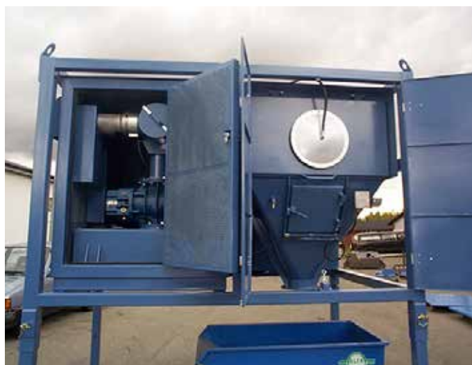
The DISAB SEBF-II vacuum unit is equipped with a mechanical safety valve that opens at the maximum vacuum.
