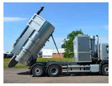
Emptying can be done by adding the function vibrators, which allow the tank to be tipped with support. The tailgate is hydraulically operated.
